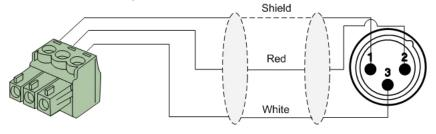
For unbalanced line output connections:
